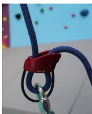
Rope correctly threaded through belay plate
